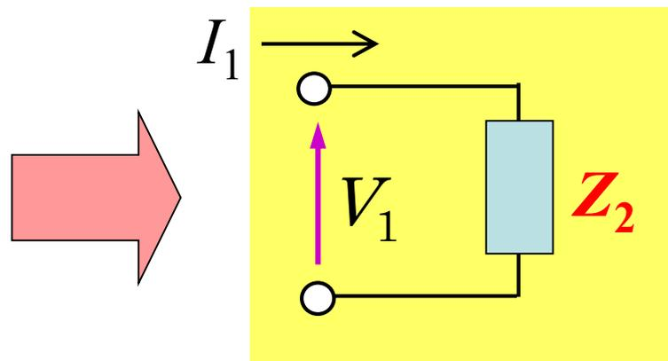
$$Z_2 = \frac{V_1}{I_1} = \left( \frac{n_1}{n_2} \right)^2 R_L$$
