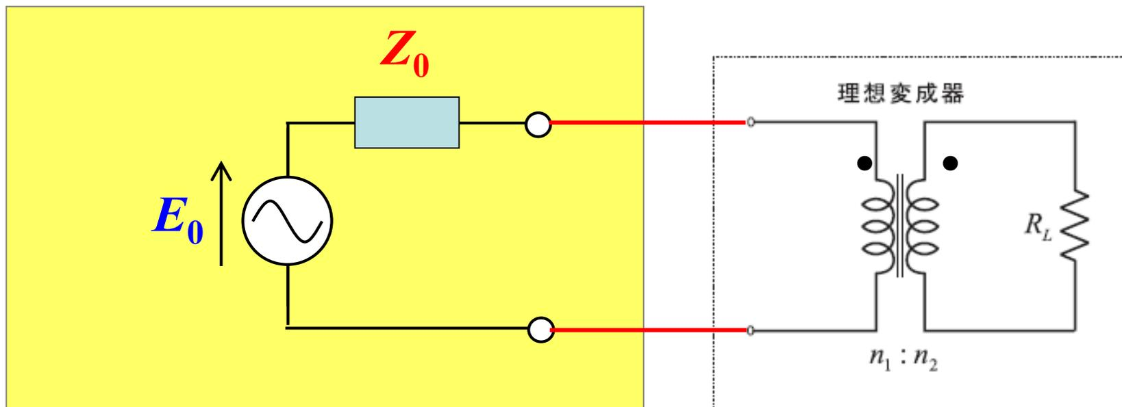
$$\left\{ \begin{array}{l} E_0 = \frac{1}{\sqrt{2}} \frac{1}{1 + j\left(\frac{\omega}{2} - \frac{1}{\omega}\right)} \\ Z_0 = \frac{1}{1 + j\left(\frac{\omega}{2} - \frac{1}{\omega}\right)} = \sqrt{2}E_0 \end{array} \right.$$
