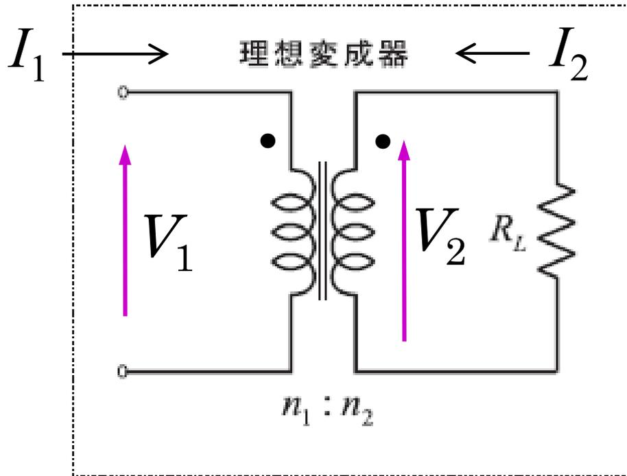
$$V_1 I_1 = V_2 I_2$$
